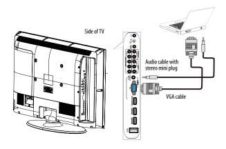
3 Connect an audio cable with stereo mini plug (not provided) to the PC IN AUDIO jack on the back of your TV and to the LINE OUT or AUDIO OUT jack on the computer.
